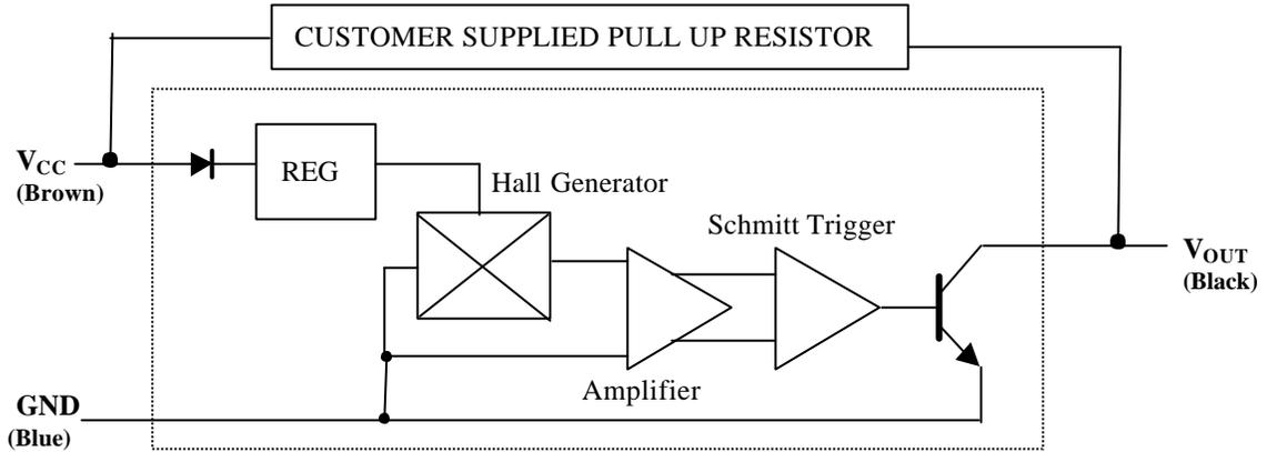
NOTE: A pull-up resistor is required on the open collector output to establish a quiescent voltage level. The pull-up resistor also provides faster rise times and improves noise immunity. Contact the factory for application assistance.
